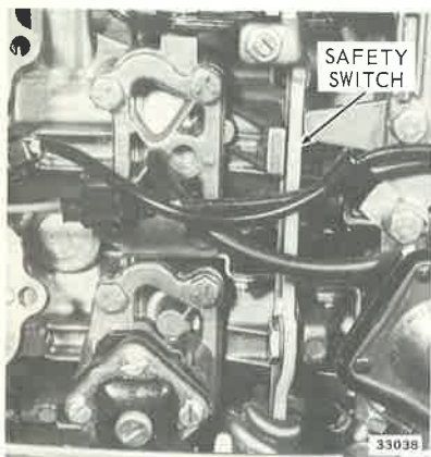
Figure 7-14. Safety Switch
