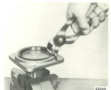
Figure 8-8. Removing Spring From Tool Base
