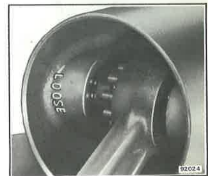
Figure 5-12. "LOOSE" Mark in Piston
