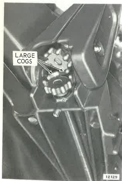
Figure 6-25. Throttle Gear Mesh
