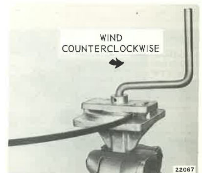
Figure 8-6. Winding In Spring
