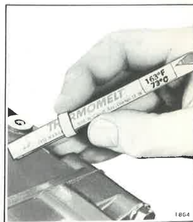
Figure 5-4. Checking Engine Temperature
