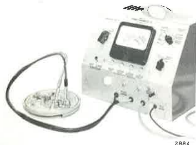
Figure 4-21. Breaker Point Testing
