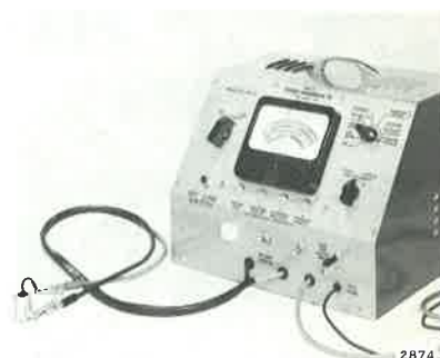
Figure 4-20. Condenser Testing
