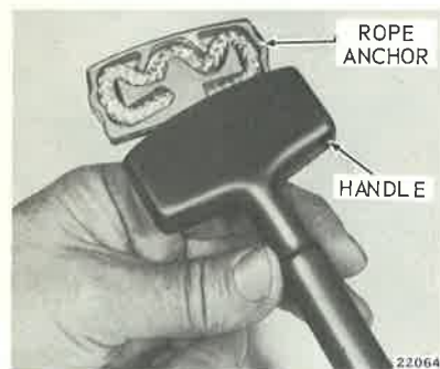
Figure 8-3. Removing Handle
