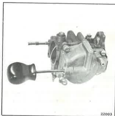
Figure 3-7. Removing Fixed Jet Orifice Plug
