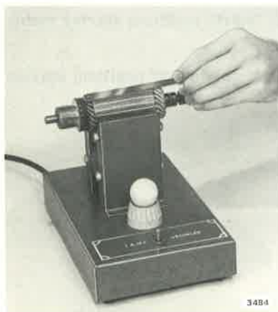
Figure 7-9. Checking Armature on Growler
