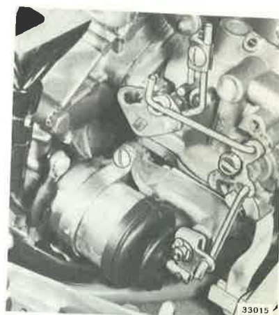
Figure 3-18A. Choke Solenoid
