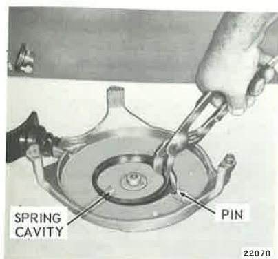
Figure 8-9. Installing Spring In Starter Housing
