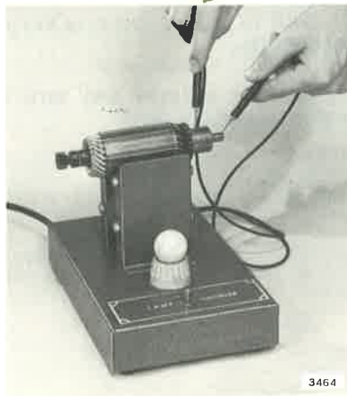
Figure 7-10. Checking Armature for Grounding
