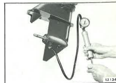
Figure 6-22. Gearcase Pressure Test
