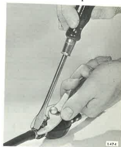
Figure 3-26. Attaching Hose Clamp
