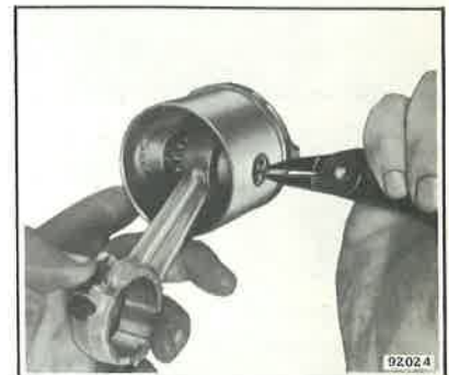
Figure 5-11. Removing Wrist Pin Retaining Ring
