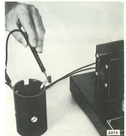
Figure 7-11. Checking Field Continuity
