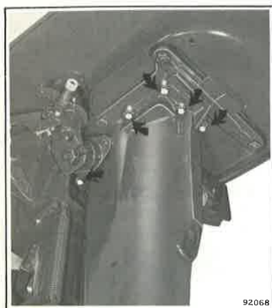
Figure 5-6. Power Head Attaching Screws
