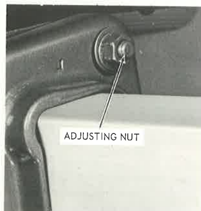
Figure 6-28. Tilt Friction Adjustment
