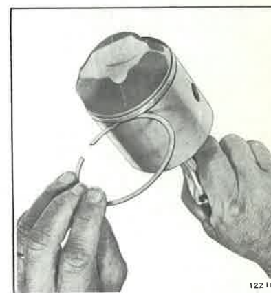
Figure 5-18. Checking Fit of Ring in Groove
