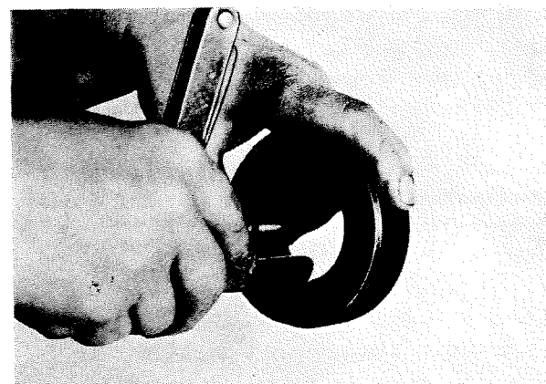
Photo 63. Setting of Piston Ring by means of standard guage
