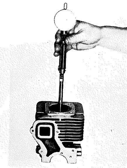
Photo 61. Measuring the Cylinder
