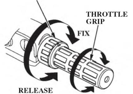
Use the throttle friction adjuster to help hold a constant throttle setting while cruising.
