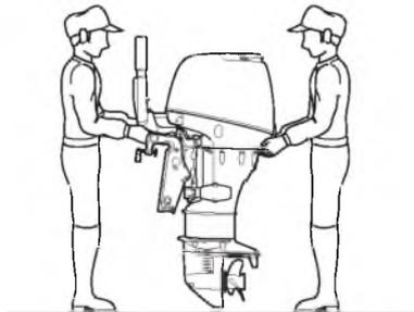
To carry, hold the outboard motor by the carrying handle, or hold by the carrying handle and the lug beneath engine cover lock lever, as shown.
