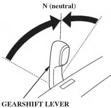
2. Check the position of the gearshift lever. It must be in the N (neutral) position for starting.
