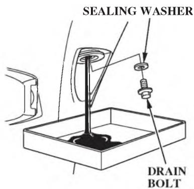
2. Place a suitable container below the drain bolt hole to catch the used oil, then remove the engine oil drain bolt and washer.
