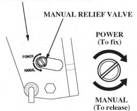
The outboard motor can also be tilted manually after opening the manual relief valve. This feature enables the outboard motor to be tilted when no battery is connected.
