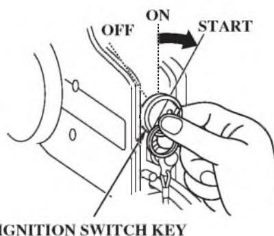
4. Turn the ignition switch key to the START position and hold it there until the engine starts.
