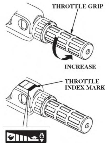
The throttle grip controls engine speed.
