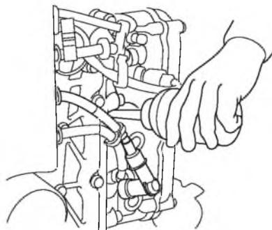
5. Pour a teaspoon of engine oil into each spark plug hole, then pull the emergency starter rope several times to lubricate the inside of the cylinders.
