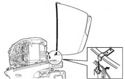
The engine cover latch fastens the engine cover to the outboard motor.
