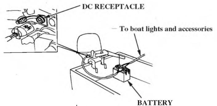
To prepare the outboard motor for connection to a battery, pull the cover off the DC receptacle, connect the battery charging wires to the plug. Attach the plug to the receptacle on the motor.
