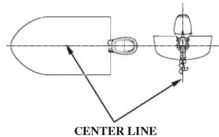
Install the outboard motor on the center of the boat transom.
