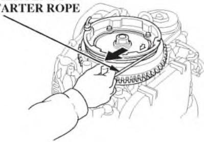
5. Pull the emergency starter rope slowly until resistance is felt, then pull briskly.
