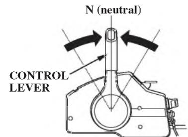
1. Move the throttle grip to the slowest speed and gearshift lever or control lever to N (neutral) position.
