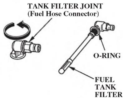
1. Unscrew the fuel hose connector by turning it counterclockwise, then remove the fuel hose connector and fuel tank filter from the tank.
