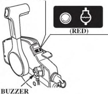
If the engine overheats, the red light will come on, and the engine protection system will limit engine speed. When normal engine temperature is restored, the engine speed will gradually rise to normal engine speed.
