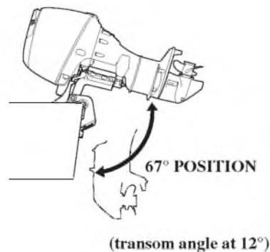
To tilt the outboard motor, move the tilt lever to the TILT position, then raise the outboard motor to the 67° position by pulling on the engine cover grip as described on p. 60.
