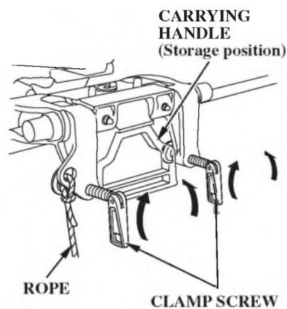
Attach the stern bracket to the boat transom by tightening the clamp screws. Push the carrying handle into the storage position. (tiller handle type)
