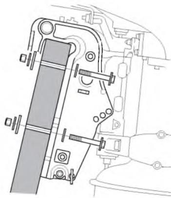
2. Secure the outboard motor with the bolts, nuts and washers.
