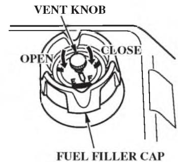
The cap is provided with a vent knob to seal the portable fuel tank for carrying it to and from the boat. Open the vent knob 2 or 3 turns before starting the engine.
