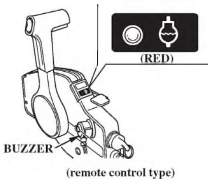
If the engine overheats, the red indicator light will come on, and the engine protection system will limit engine speed. If you are at cruising speed, engine speed will decrease gradually. When normal engine temperature is restored, the engine speed will gradually rise to normal engine speed.
