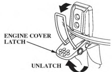
1. Unlatch and remove the engine cover.
