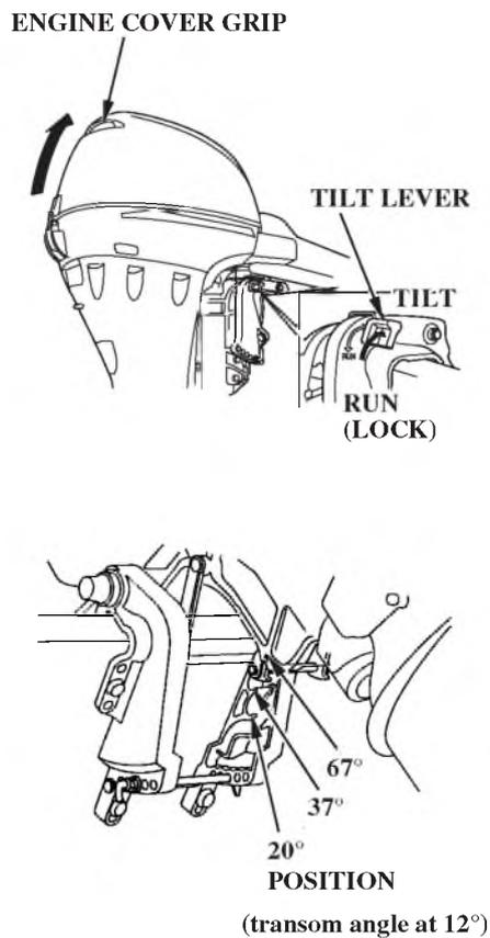
To tilt the outboard motor, move the tilt lever to the TILT position, then raise the outboard motor to the 20° or 37° position by pulling on the engine cover grip.
