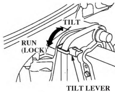
The tilt lever enables the outboard motor to be raised for shallow water operation, beaching, launching, or mooring.
