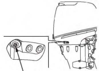
Water should flow from the cooling system indicator while the engine is running. This shows that water is circulating through the cooling system.
