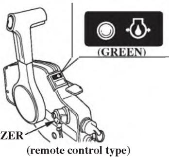
If oil pressure becomes low, the green indicator light will go off, and the engine protection system will limit engine speed. If you are at cruising speed, engine speed will decrease gradually.
