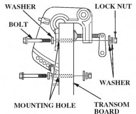
You may further secure the outboard motor by bolting the stern bracket to the boat transom. Use the optional mounting bolt and nut kit or other good quality stainless steel bolts, nuts, and washers. Apply silicone sealant to the bolt holes.
