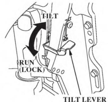
Moving the tilt lever to the TILT position allows the outboard motor to be tilted and moving the tilt lever to the RUN (LOCK) position locks the outboard motor in the desired position. Use the tilt lever to temporarily tilt the outboard motor when the boat is operating in shallow water, or mooring in shallow water. The tilt lever must be in the RUN (LOCK) position before operating the outboard motor or the motor could tilt up when operating in reverse.
