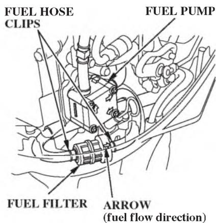
6. Install the new fuel filter so the arrow on the filter points toward the fuel pump.
