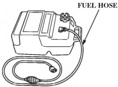
Empty the portable fuel tank into an approved gasoline container. Use a funnel to avoid spilling fuel. Rinse the fuel tank with nonflammable solvent to remove any accumulated sediment.
